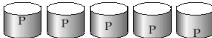
(f) RAID 5: block-interleaved distributed parity
